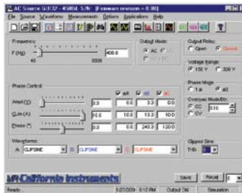
Soft front panel control through Windows GUI.
