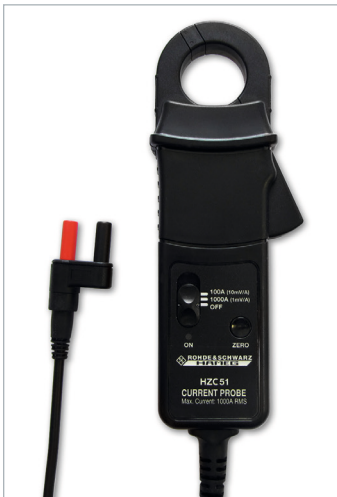
HZC51 AC/DC current probe.
