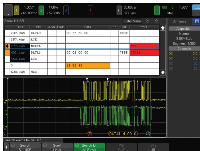
Figure 21. USB 2.0 trigger, decode and "lister" display.
