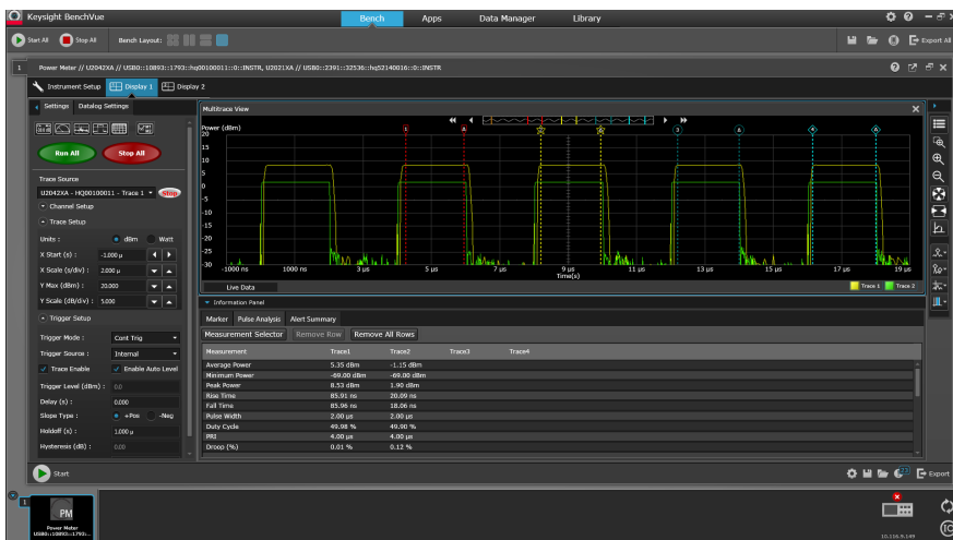
Figure 9. Multi-channel trace display with 4-pairs of gates and automatic pulse parameters measurement (sample screen shot with two U2042XAs).
