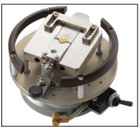
TO workholder with mechanical clamping
