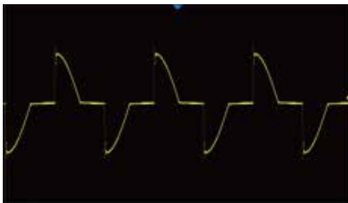
LeadingEdge phase dimming
