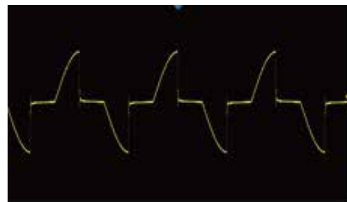
TrailingEdge phase dimming
